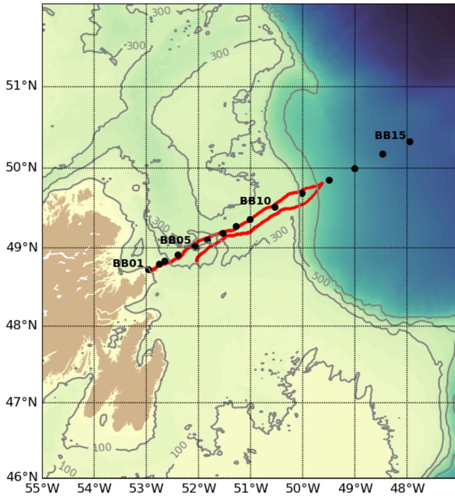
FIGURE 1 – Bathymetric map of the region, including the hydrographic stations on the Bonavista Section (black circles) and the glider track (854 casts in red).
